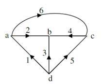
10. (a) Define and state the properties of incidence matrix.[L2] [4M](b) For the network shown below draw the graph and find incidence and tie – set matrices.
